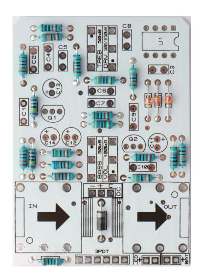
Place the resistors and diodes. If you have troubles reading the values, check out our "Reading Part Values" tutorial.
