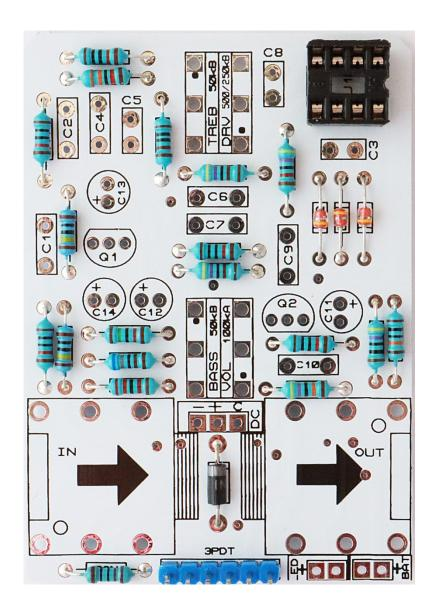
Then, solder the IC sockets (without the ICs) and the pin header.
